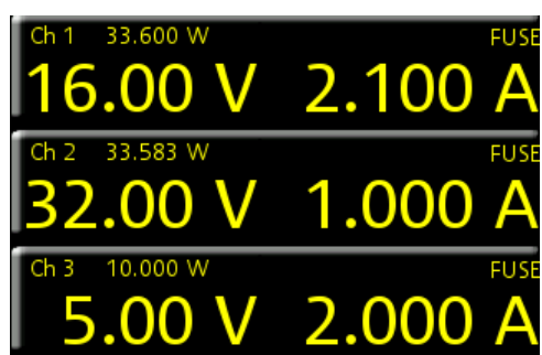
Figure 5-11: Fuse switched on for the respective channel
