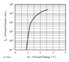
Figure 4. Forward Current vs. Forward Voltage
