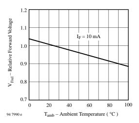
Figure 5. Relative Forward Voltage vs. Ambient Temperature
