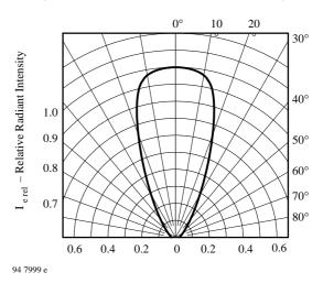
Figure 10. Relative Radiant Intensity vs. Angular Displacement
