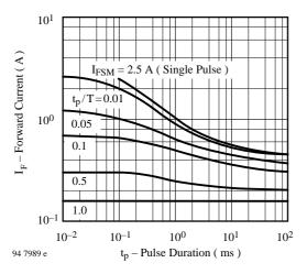
Figure 3. Pulse Forward Current vs. Pulse Duration
