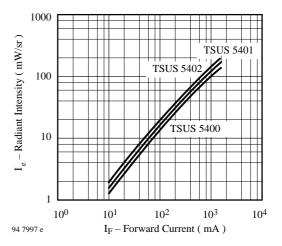
Figure 6. Radiant Intensity vs. Forward Current
