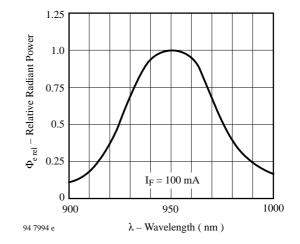
Figure 9. Relative Radiant Power vs. Wavelength
