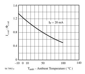
Figure 8. Rel. Radiant Intensity\Power vs. Ambient Temperature
