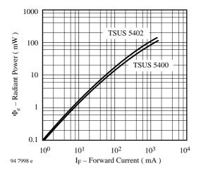
Figure 7. Radiant Power vs. Forward Current
