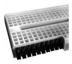
Depending on the size and arrangement of the clips, we get either a socket strip or a bus strip. The socket strip is used for connecting components together. It has two rows of short (5 contact) clips arranged one above another, like this:
