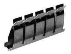
The clip is made of nickel silver material which is reasonably conductive, reasonably springy, and reasonably corrosion resistant. Because each of the pairs of fingers is independent we can insert the end of a wire between any pair without reducing the tension in any of the other fingers. Hence each pair can hold a wire with maximum tension.
