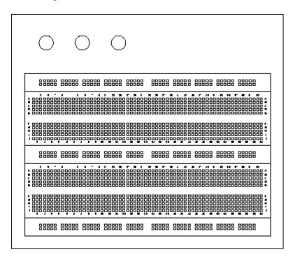
In this picture we have replaced the plastic covers, hiding the connections The breadboard lets us connect components together and by wiring the bus strips to the binding posts and the binding posts to the power supply, to connect the power supply to the circuit. Now what we need is a way to bring connections from the rest of the instruments into the breadboard.
